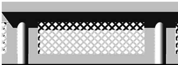
Elevation with bold pattern lattice screen panel.
